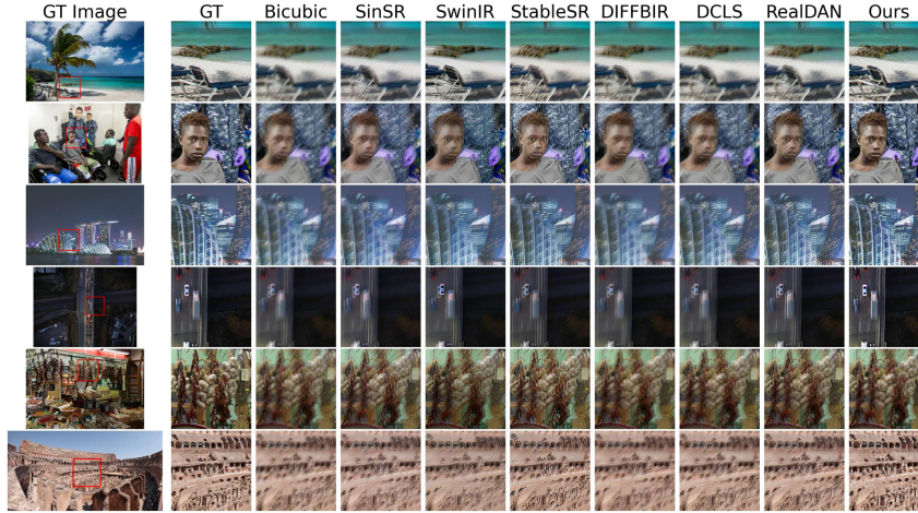
Figure 3: Blind-SR comparison on the DIV2KFK dataset (4 \times SR). Each row relates to a different LR image from DIV2KFK, while each column shows the output of a different method. Notably, our method reduces doubling artifacts in structured patterns (e.g., aerial road scene, 4th row), demonstrating its effectiveness in restoring fine details and mitigating motion effects.
